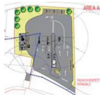
Fig. 10 Hydrogen refueling Station preliminary design
